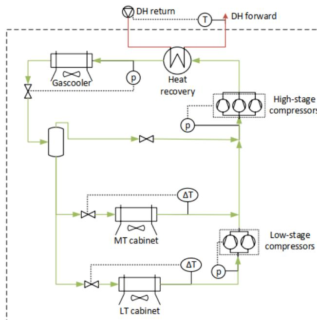
Figure 2: Scheme of CO<sub>2</sub> refrigeration system and waste heat utilisation with heat exchangers [17]
