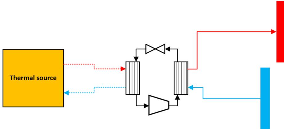
Figure 88 Thermal source connection – heat pump configuration
