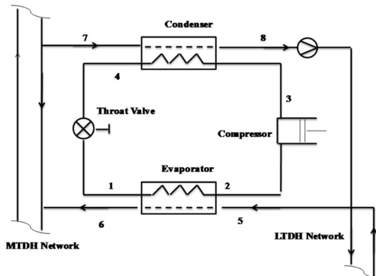
Figure 16 - Integration of medium temperature DH and low-temperature subnetwork with HP [41]
