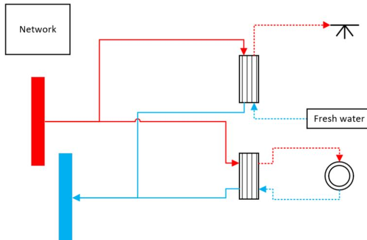
Figure 67 LTDH substation – Instantaneous heat exchanger unit
