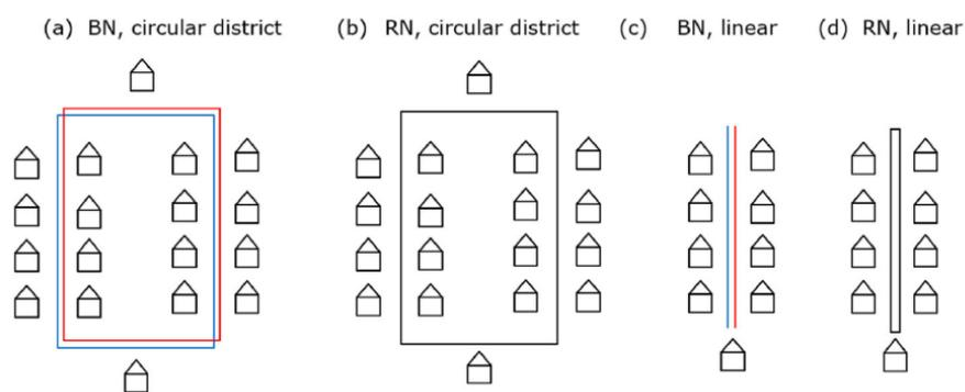
Figure 42 Overview of “traditional” two-pipe and one-pipe “reservoir” NTDH network topologies [60]
