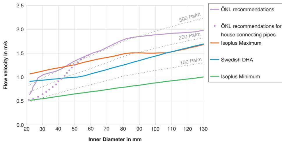
Figure 36 Maximum flow velocities for different pipe sizes and specific pressure losses optimal economic operation of the DH network [55]
