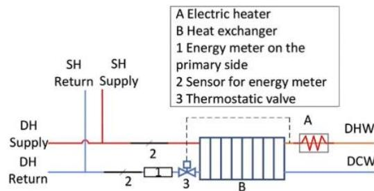
Figure 55 ULTDH substation based on electrical heaters on kitchen taps [65]
