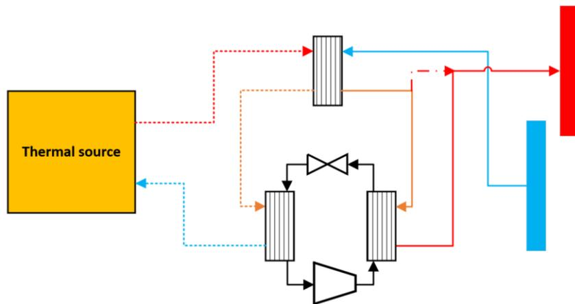
Figure 89 Thermal source connection – heat exchanger and heat pump configuration
