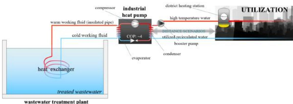
Figure 9: Scheme of the wastewater utilization in the district heating systems [34]
