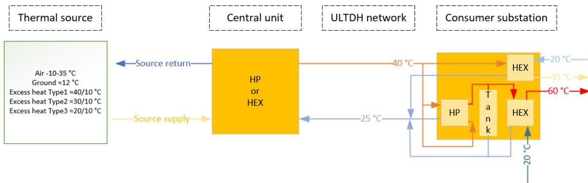
Figure 91 ULTDH network-based system with booster heat pump substation
