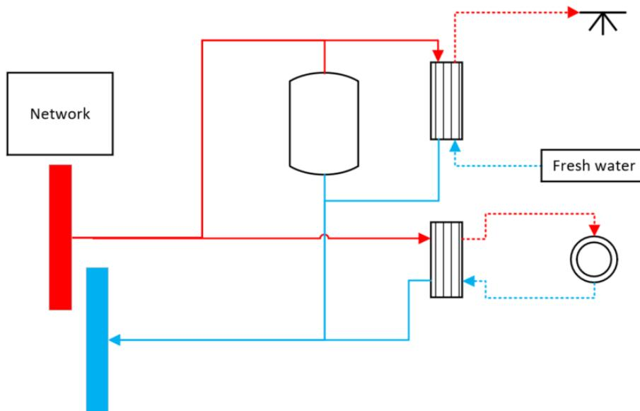
Figure 68 LTDH substation – District heating storage unit
