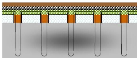
Figure 23 Borehole thermal storage overview
