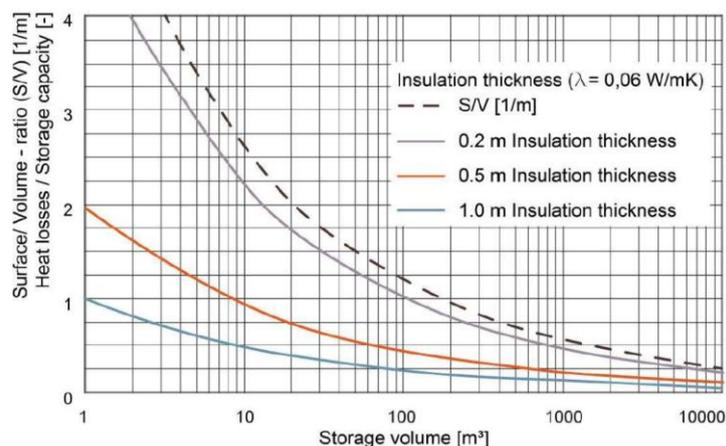
Figure 29 Heat losses and storage volume correlation
