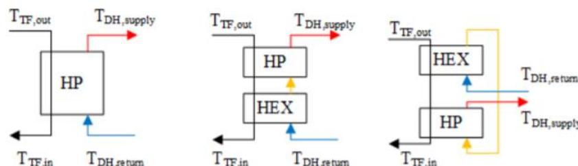
Figure 6: Configuration for the possible waste heat recovery systems of the transformer [27]
