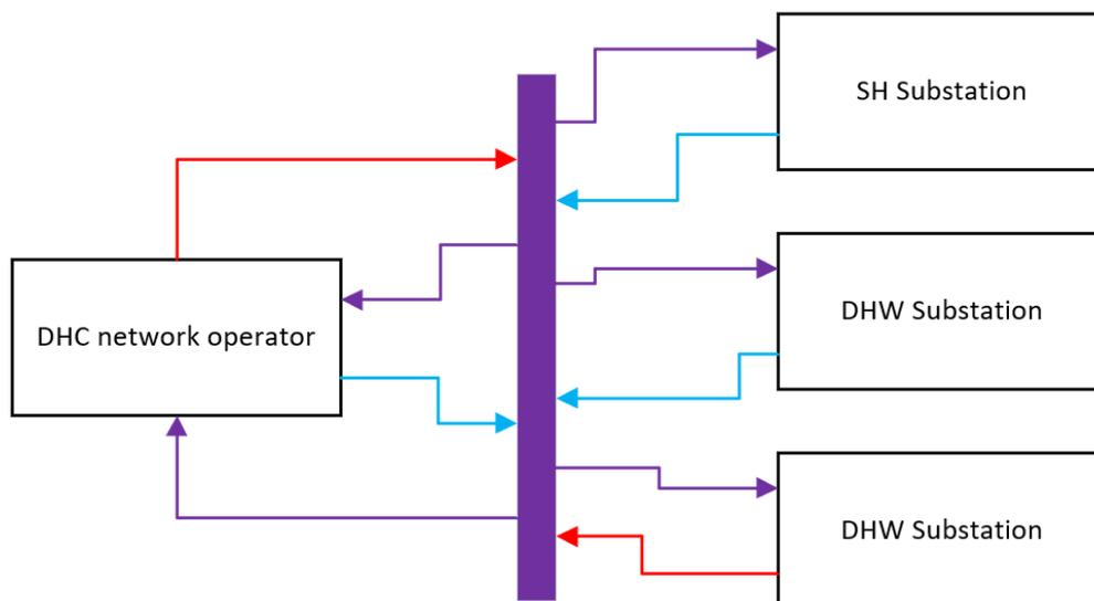
Figure 84 Thermal network – 1-pipe network for SH, SC and DHW (reservoir network)
