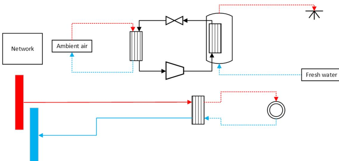
Figure 72 ULTDH substation – other booster technology (e.g. air heat pump)
