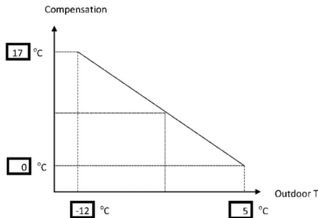
Figure 34 Supply temperature compensation in ULTDH networks [49]
