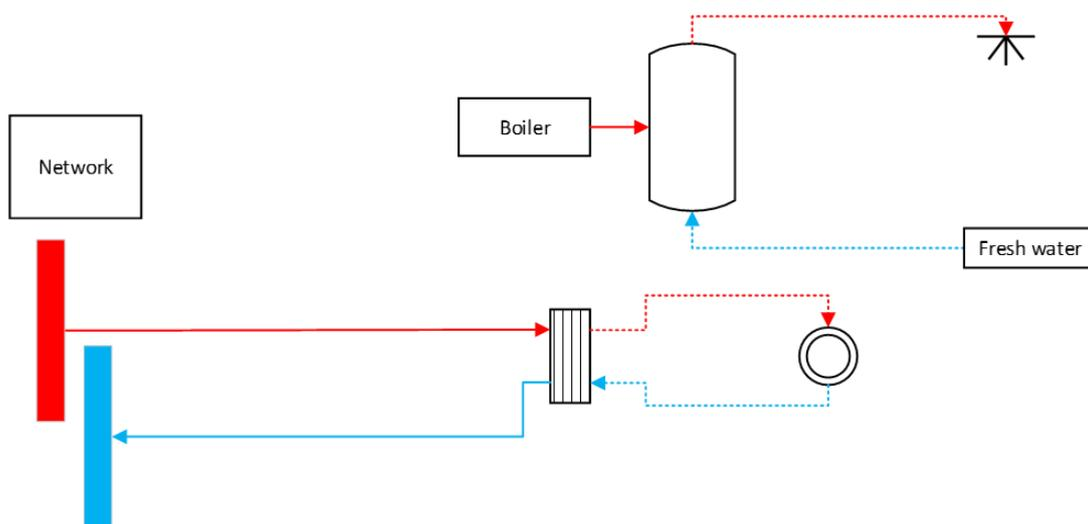
Figure 73 ULTDH substation – other booster technology (e.g. boiler)
