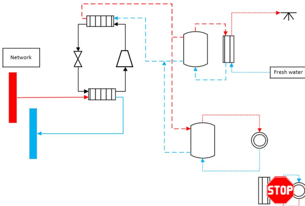
Figure 75 NTDH substation – BHP for DHW and SH, SC as heat source for DHW BHP (heating mode)
