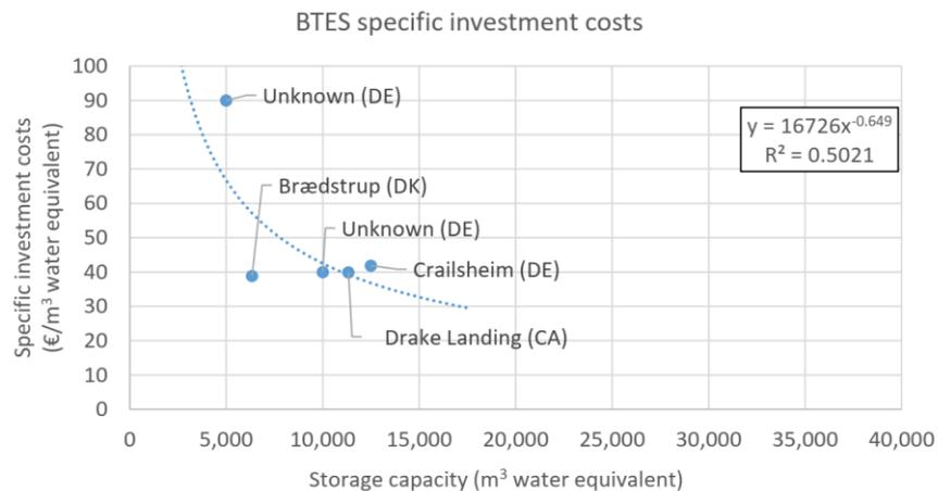
Figure 24 Borehole thermal storage specific investment
