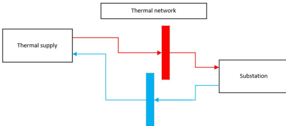
Figure 80 Thermal network – 2-pipe “traditional” network
