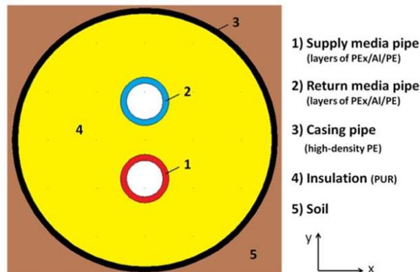
Figure 31 - Geometry and materials of a flexible, pre-insulated, twin pipe [42]
