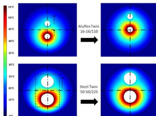
Figure 33 - Proposed modification in DH pipe design (IEA DHC, 2014.)
