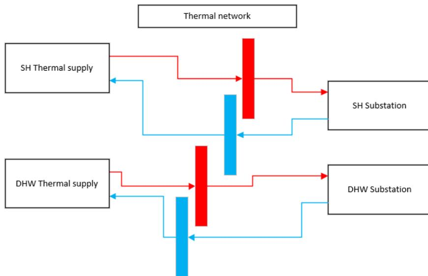
Figure 81 Thermal network – 4-pipe network for SH/SC and DHW (heating mode)
