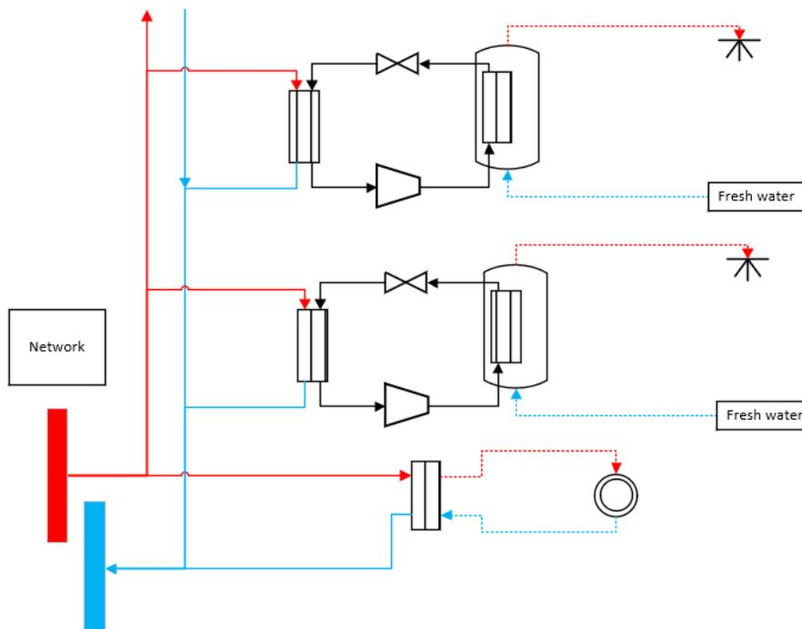
Figure 71 ULTDH substation – micro booster heat pumps
