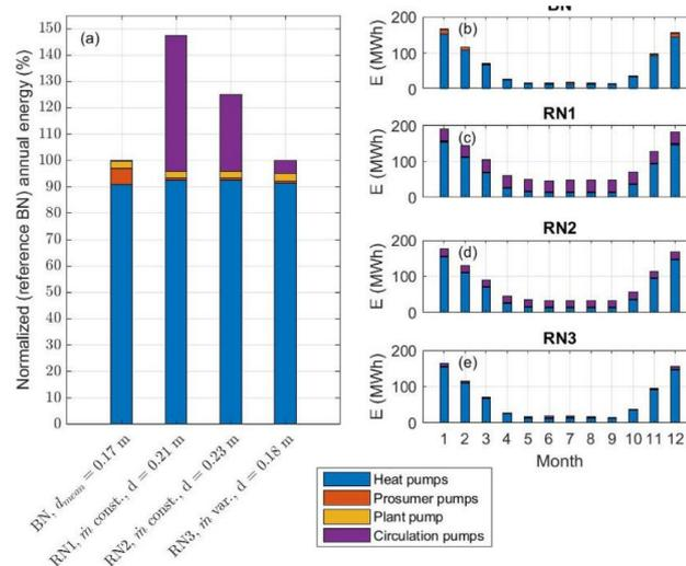
Figure 43 Pumping power consumption for different NTDH topologies and system controls
