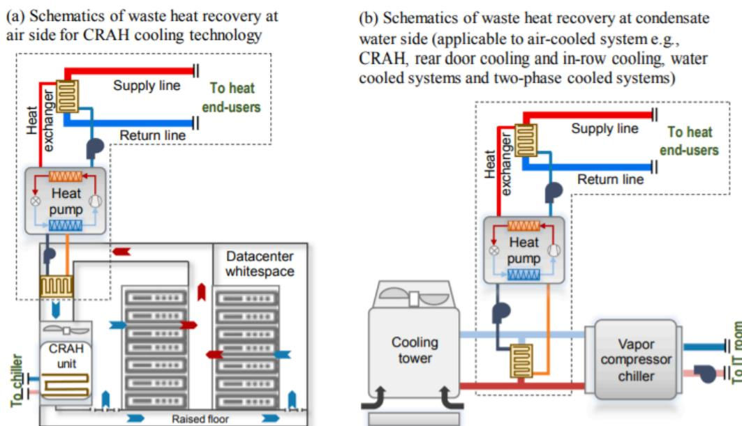
Figure 5: Schematic diagram of the heat reuse solutions – on the left schematic of waste heat recovery at air side for CRAH cooling technology; on the right schematic of waste heat recovery at the condensate water side
