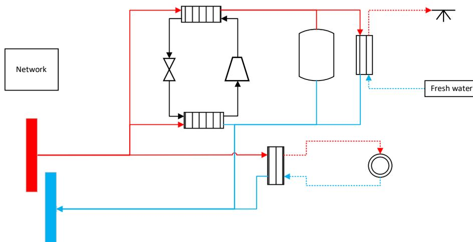
Figure 69 ULTDH substation – booster heat pump (supply split to evaporator and condenser) and district heating storage unit
