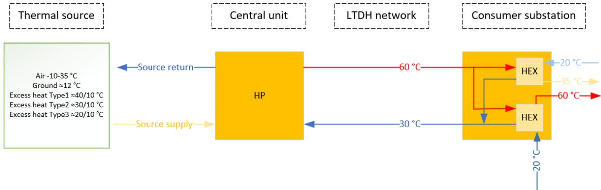
Figure 90 LTDH network-based system with district heating storage unit substation
