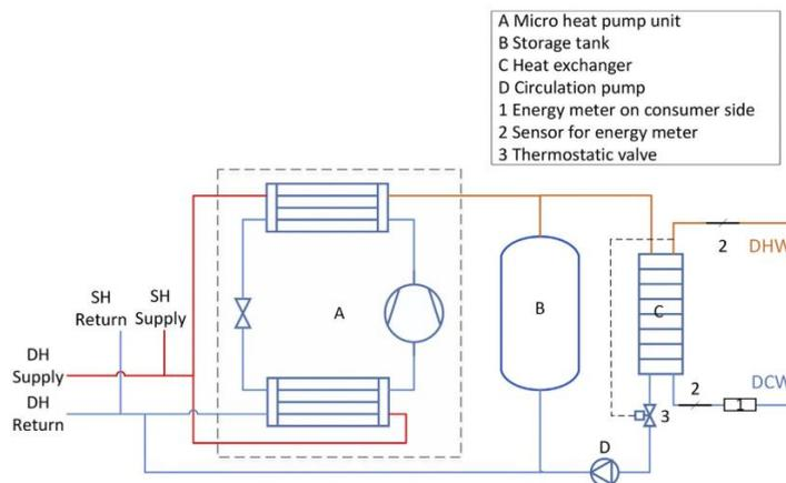
Figure 53 ULTDH substation based on heat pump [65]
