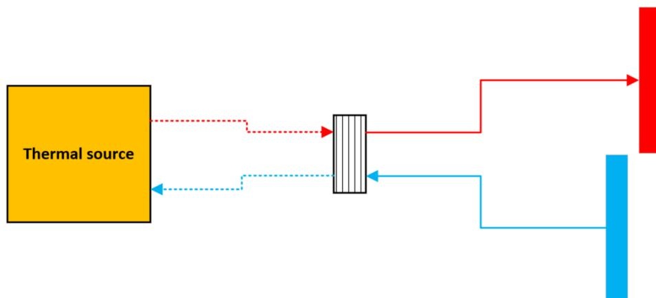
Figure 87 Thermal source connection – heat exchanger configuration
