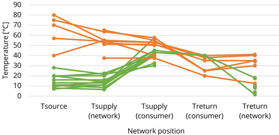
Figure 64 Temperature levels across DH system: green - NTDH, orange - LTDH
