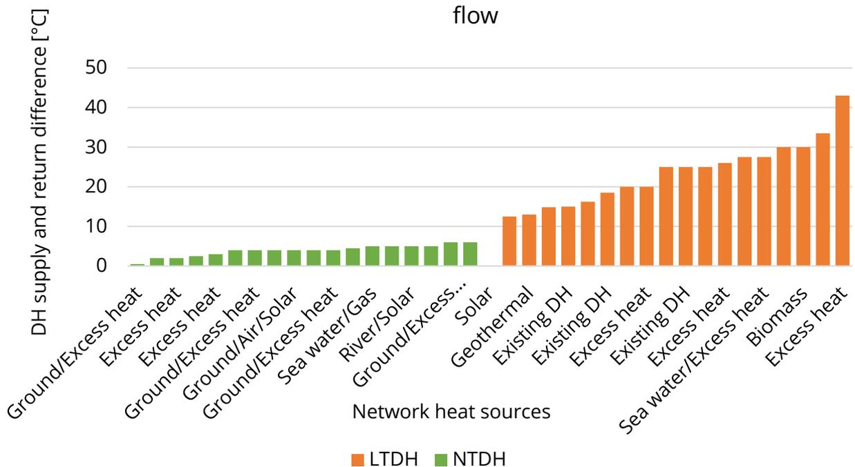
Figure 65 DH network supply and return temperature for different systems
