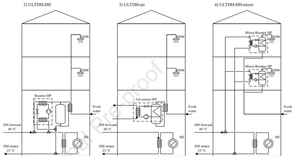
Figure 50 Different ULTDH substations for DHW production [4]
