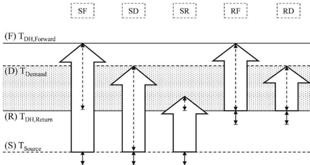
Figure 18 Different heat pump configurations in district heating system
