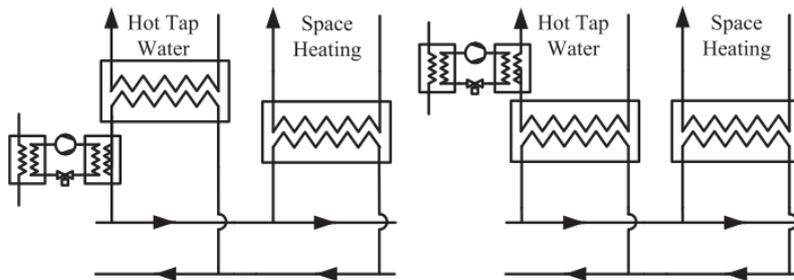
Figure 49 Booster heat pump positioning in a DHW preparation system [5]
