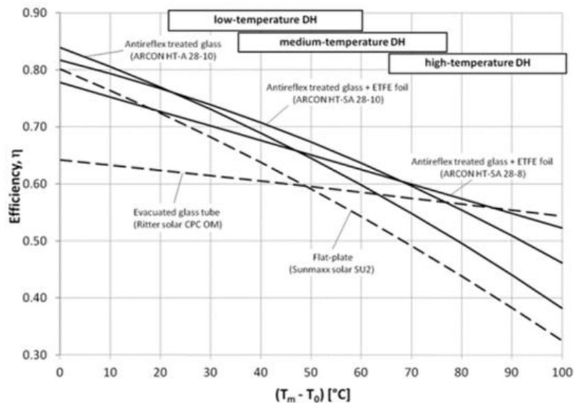
Figure 12 Efficiency of solar collector as a function of the difference between the mean collector fluid and ambient temperature [42]
