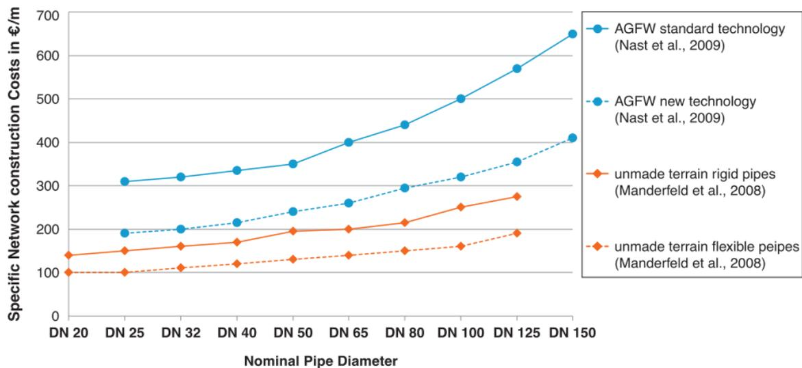
Figure 38 Specific network construction cost for different pipe sizes [55]
