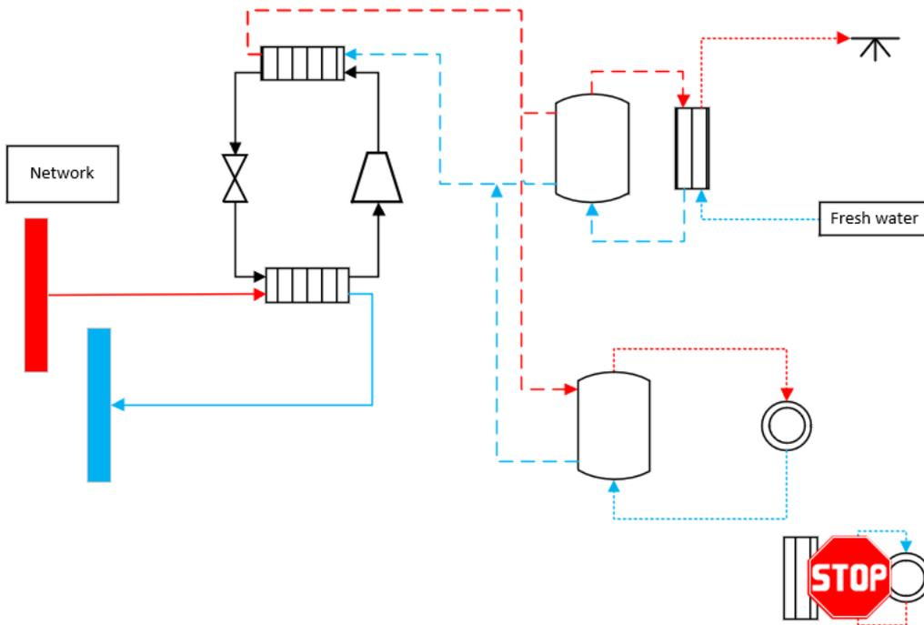
Figure 77 NTDH substation – reversible heat pump for SH/DHW and SC (heating mode)
