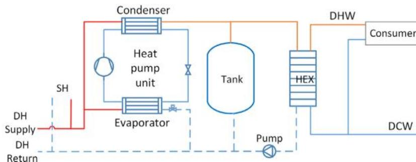
Figure 48 Heat pump booster unit in combination with tank on the primary side [63]
