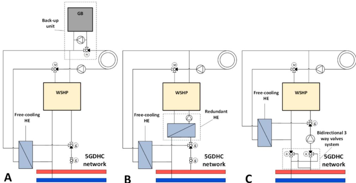
Figure 57 Proposal of NTDH substation by Buffa et al [56]
