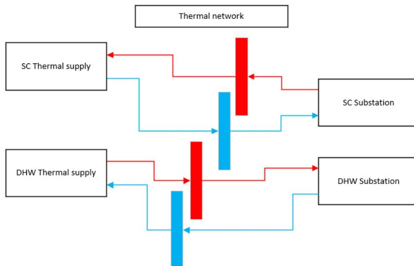
Figure 82 Thermal network – 4-pipe network for SH/SC and DHW (cooling mode)
