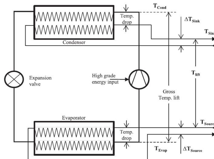
Figure 17 Overview of heat pump cycle and temperature levels [46]
