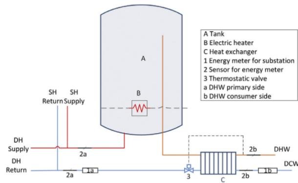
Figure 52 ULTDH substation based on district heating storage tank [65]
