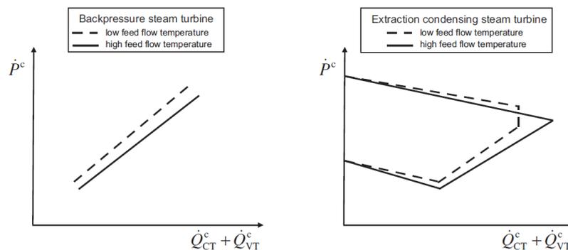
Figure 10 P-Q diagrams of different CHP types and the impact of DH network temperature reduction [37]
