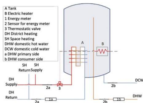
Figure 51 ULTDH substation based on immersion heater [65]
