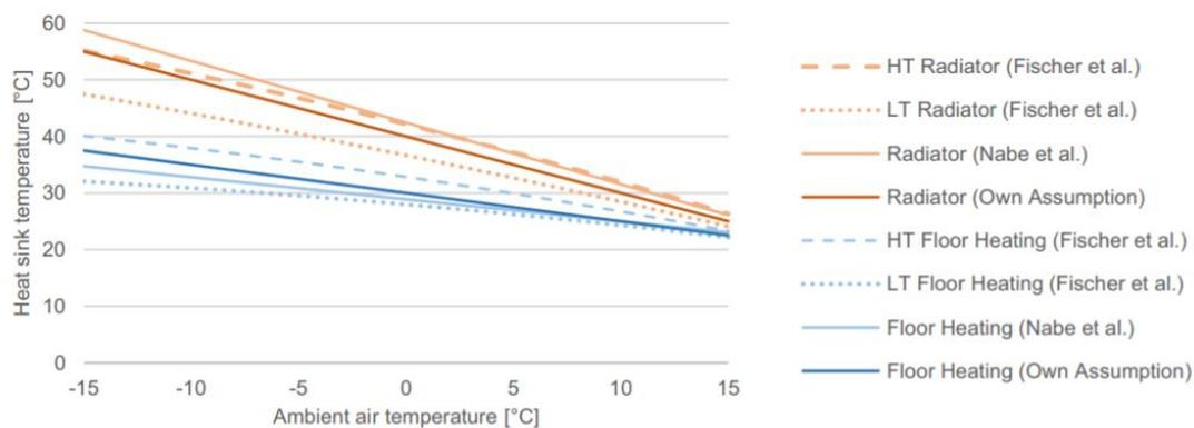
Figure 44 Different space heating temperature regimes [61]
