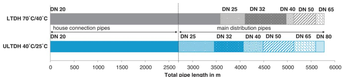
Figure 37 Different pipe size for LTDH and ULTDH network [55]
