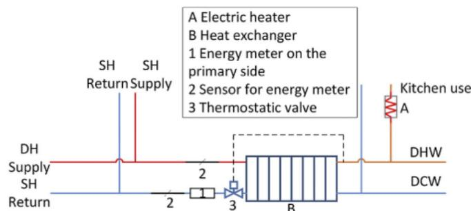
Figure 54 ULTDH substation based on electrical heaters on kitchen taps [65]
