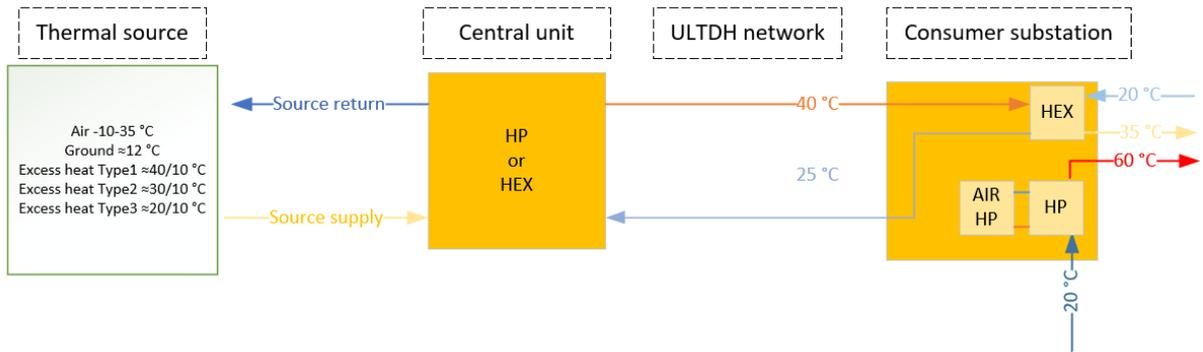
Figure 93 ULTDH network-based system with air-source heat pump substation
